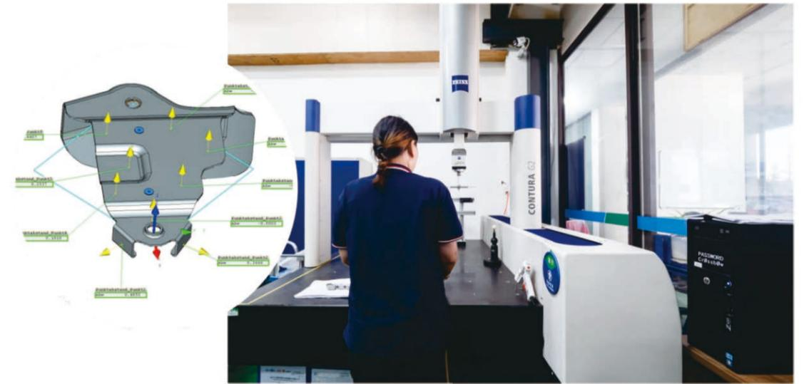
All these precision inspection instruments can ensure the quality control in every project process including material incoming check, individual tool components inspection, cut-off samples measurement etc.
